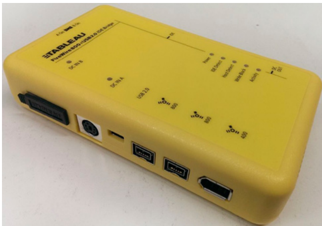
Figure 2. A read-write capable write-blocker
